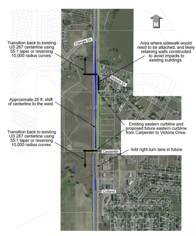
Figure 6-2: Alignment Shift at Carpenter Road
