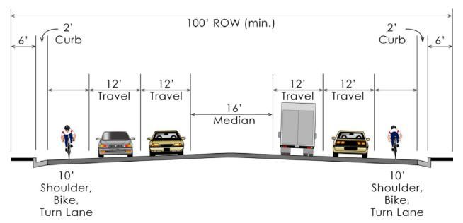
Figure 3-7: Existing US 287 Cross Section
